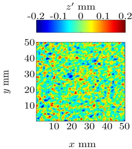
Figure 3 : Surface roughness scan result
