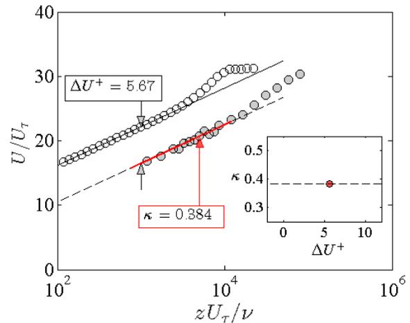
Figure 3: Mean velocity profile of smooth wall (from Marusic et al [19] ), marked with open circles; and the rough ship hull , marked with grey circles. The inset figure shows the value of Hama roughness function against  $\kappa$ .
