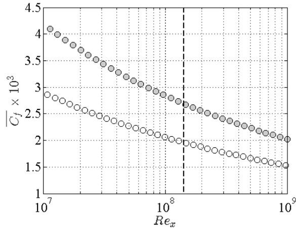
Figure 4: Average skin friction coefficient against Reynolds number for the (open circles) smooth surface and (grey circles) for the rough surface from LDA. The vertical dashed black line is the Reynolds number of the ship at downstream location of 25.5 m (optical access location) and cruise speed of 5 m/s
