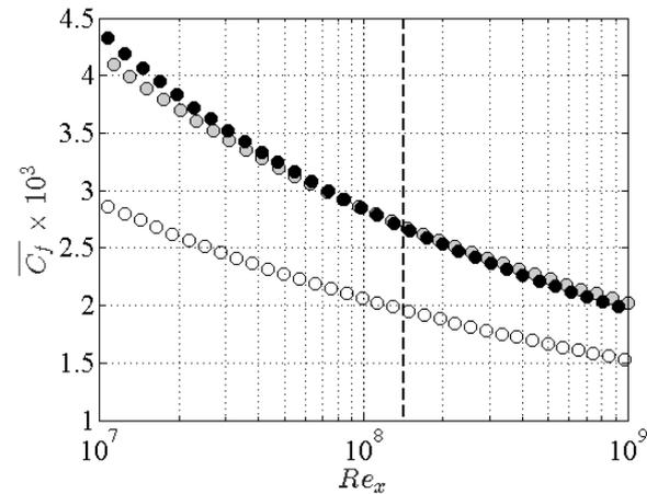
Figure 5: Average skin friction coefficient against Reynolds number for the (open circles) smooth surface, (grey circles) for the rough surface from LDA, and (black circle) empirical estimation. The vertical dashed black line is the Reynolds number of the ship at downstream location of 25.5 m (optical access location) and cruise speed of 5 m/s
