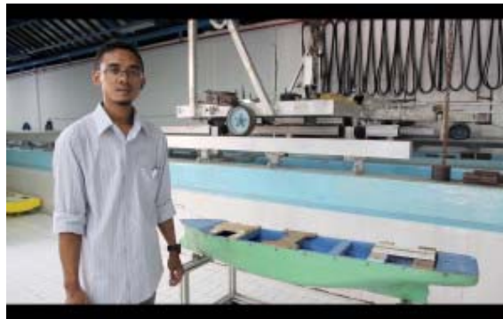
Investigating how water flows around a ship while clean, or coated in algae and barnacles, will help show where energy is being wasted. Credit: Nadia Astari
